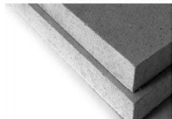
**Knauf Vidiwall is a gypsum fibreboard manufactured from gypsum and cellulose fibres from recycled paper. This dense sheet material is suitable for all areas of drywall construction requiring a dense, impact resistant product capable of providing increased durability, rigidity and mechanical strength compared to a traditional gypsum sheet plasterboard.**
