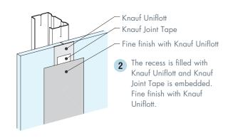
Adjacent Knauf Vidiwall boards should be closely butted together. Apply Knauf Uniflott in the stepped beveled edge and embed joint tape into it.
